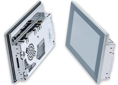
Another aspect in favor of the „Santaro 7 inch boxed“ system is its ability to be integrated perfectly into the planned bioreactor. The standard assembly was used except for the glass panel, but the 3-mm thick, chemically hardened glass was adapted. The customer’s logo was printed on the back side and it has a white border instead of black.
