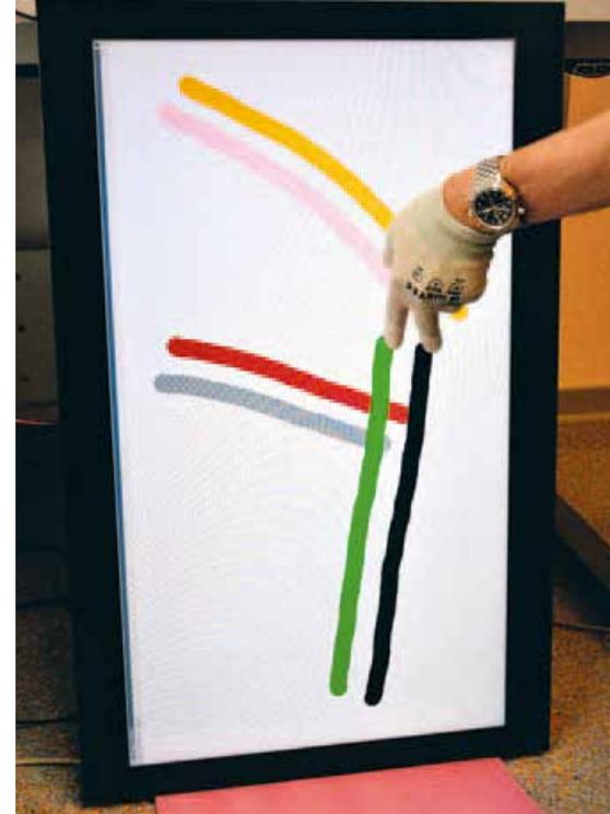
**Figure 1. Targeted programming is able to optimize a touchscreen to specific types of gloves.**
